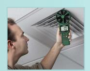
Extech's 4" (10cm) Large Vane Thermo-Anemometer series allows for more precise readings on larger size ducts. Each meter simultaneously displays Airflow or Air Velocity and Temperature. Choose models that also measure Air Volume, Humidity & Carbon Dioxide (CO<sub>2</sub>).
